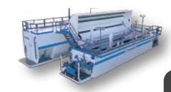
Specifically designed and engineered to handle and clean heat exchangers experiencing extreme hydrocarbon fouling at Upgraders, SAGD and Refinery operations. It can handle heat exchangers 30 feet long and 78 inches in diameter with a weight of 60,000 lbs. Cleaning is complete with minimum worker exposure and effectively cleans shell side and tube side simultaneously.
